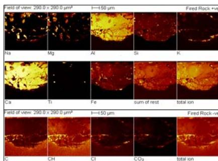
Of interest is the presence of K on the burnt crust and within the fissures. The presence of K has been attributed directly to the firing, resulting from the ash residue that would remain after firing with timber. This would not be expected if gasoline had been used for the firing.
